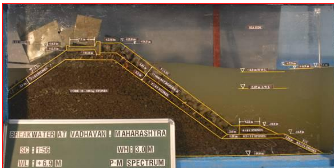
Photo-18: Wave action on trunk section armour layer (11 Cu.m Accropode-II) at -19.0m bed level with wave height of 3.0 m at +6.9 m water level
