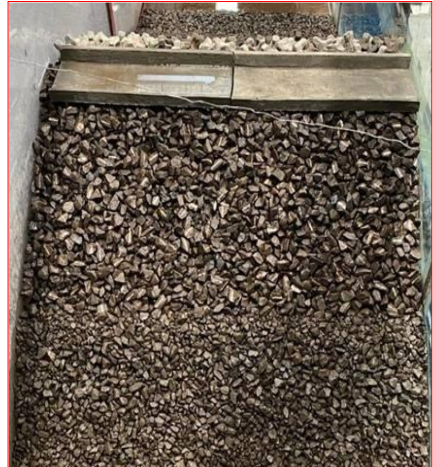
a) About 1% damage, water level of + 7.9 m, wave height of 7.0 m ( H_s ), b) About 1% damage, water level of + 6.9 m, wave height of 7.5 m ( H_s )
