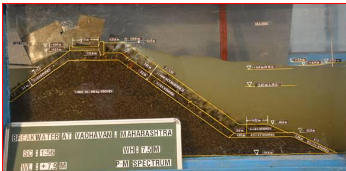
Photo-16: Wave action on trunk section armour layer (11 Cu.m Accropode-II) at -19.0m bed level with wave height of 7.5 m at +7.9 m water level
