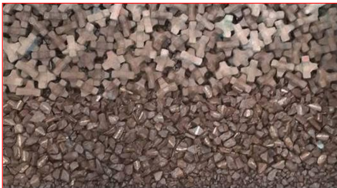
Photo-31: Toe-berm portion of breakwater section after wave generation (water level of + 0.0 m, wave height of 7.5 m ( H_s ))
