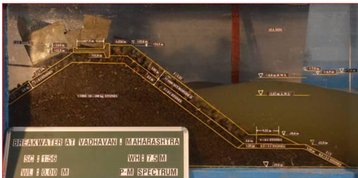
Photo-22: Wave action on trunk section armour layer (11 Cu.m Accropode-II) at -19.0 m bed level with wave height of 7.5 m at 0.0 m water level
