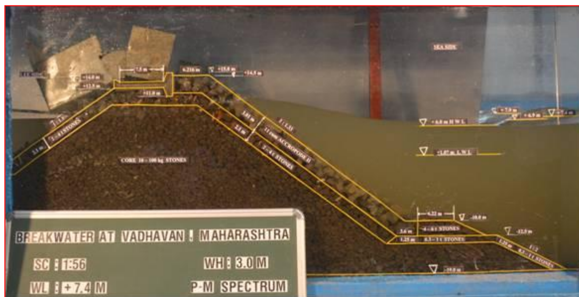
Photo-18: Wave action on trunk section armour layer (11 Cu.m Accropode-II) at -19.0m bed level with wave height of 3.0 m at +6.9 m water level
