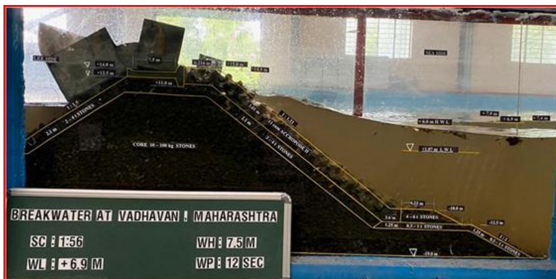
Photo-12 : Wave action on trunk section armour layer(11 Cu.m Accropode-II) at -19.0m bed level with wave height of 7.5 m at +6.9 m water level
