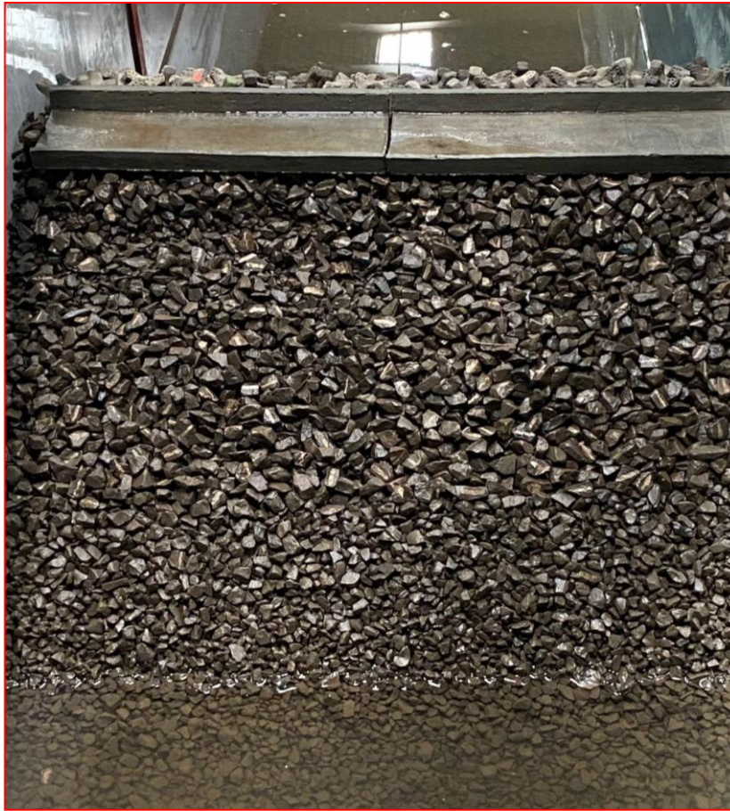
a) About 1% damage, water level of + 7.9 m, wave height of 7.0 m ( H_s ), b) About 1% damage, water level of + 6.9 m, wave height of 7.5 m ( H_s )
