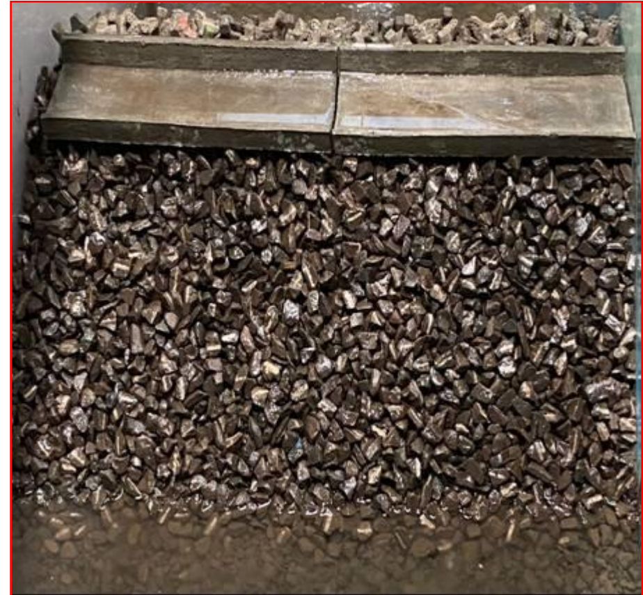
b) less than 1% damage, water level of + 7.4 m, wave height of 7.0 m ( H_s )
