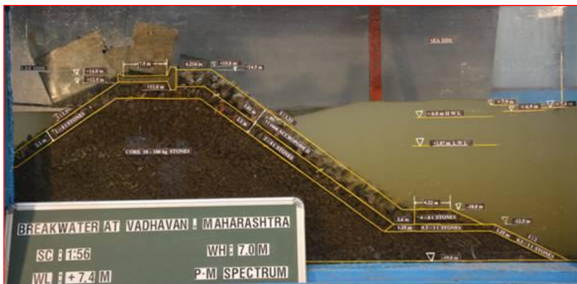
Photo-10: Wave action on trunk section armour layer (11 Cu.m Accropode-II) at -19.0m bed level with wave height of 7.0 m at +7.4 m water level
