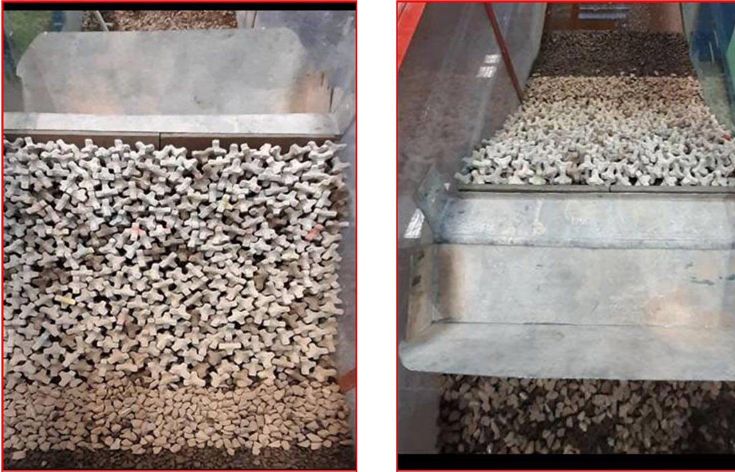
Photo-7 : Overtopping discharge tray provided in the wave flume for collection of volume of Overtopping discharge during the test
