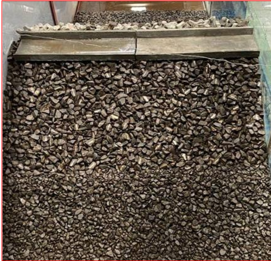
a) No damage, water level of + 6.9 m, wave height of 7.0 m ( H_s ),
