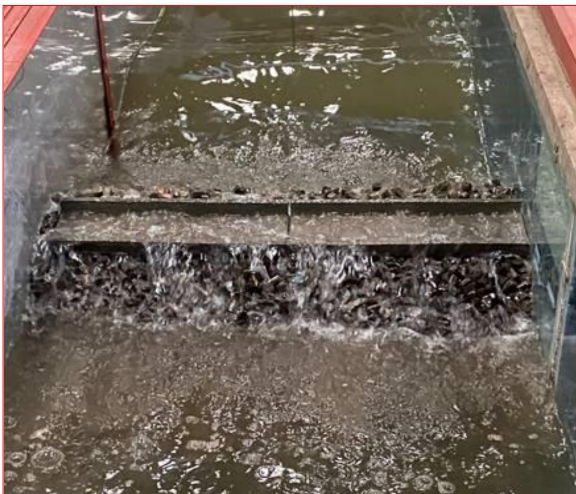
Photo-25: Overtopping of waves on leeside of breakwater section in the wave flume after wave generation
