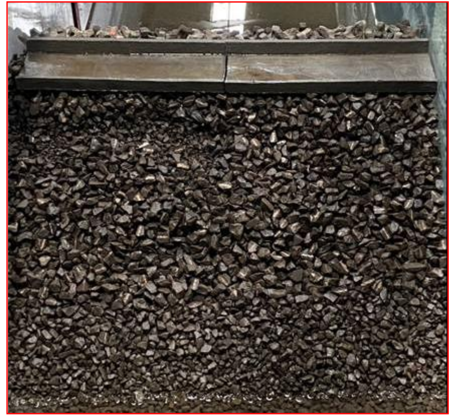
a) 3% damage, water level of + 7.4 m, wave height of 7.5 m ( H_s ), b) 5% damage, water level of + 7.9 m, wave height of 7.5 m ( H_s )
