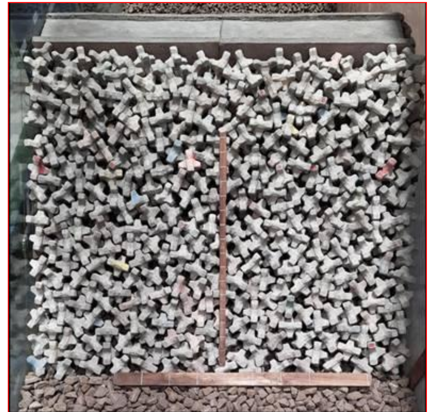
Photo-5 : Placement of Accropode™ II model units in the wave flume
