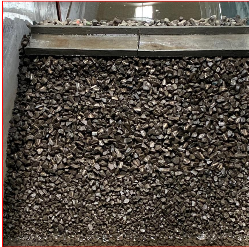
a) 3% damage, water level of + 7.4 m, wave height of 7.5 m ( H_s ), b) 5% damage, water level of + 7.9 m, wave height of 7.5 m ( H_s )
