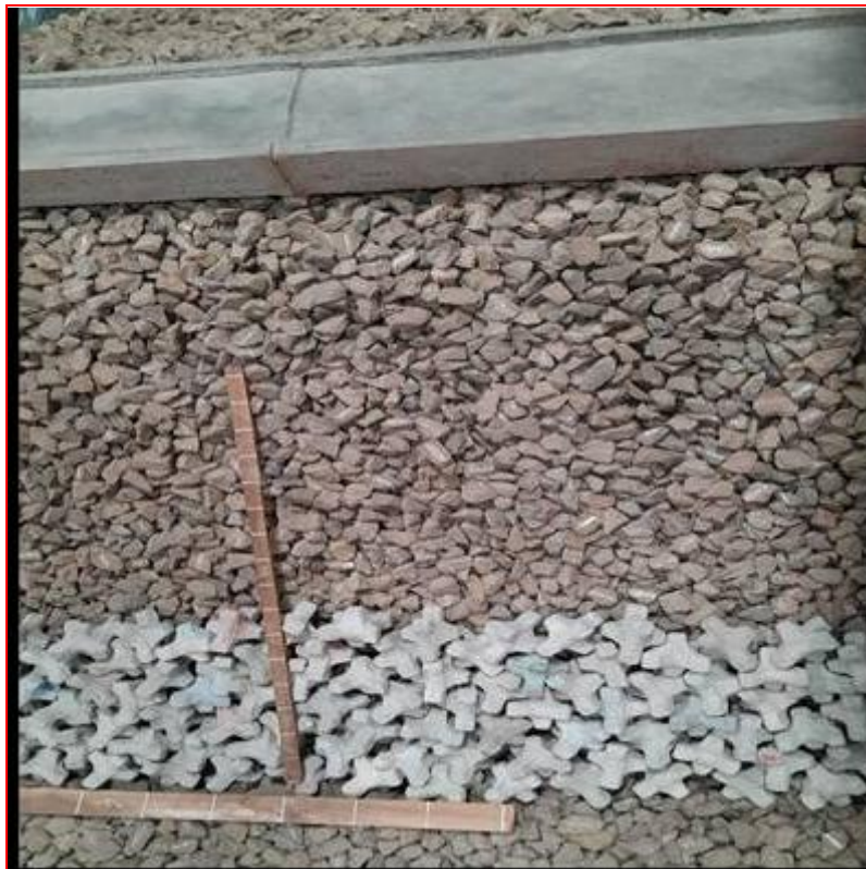
Photo-5 : Placement of Accropode™ II model units in the wave flume
