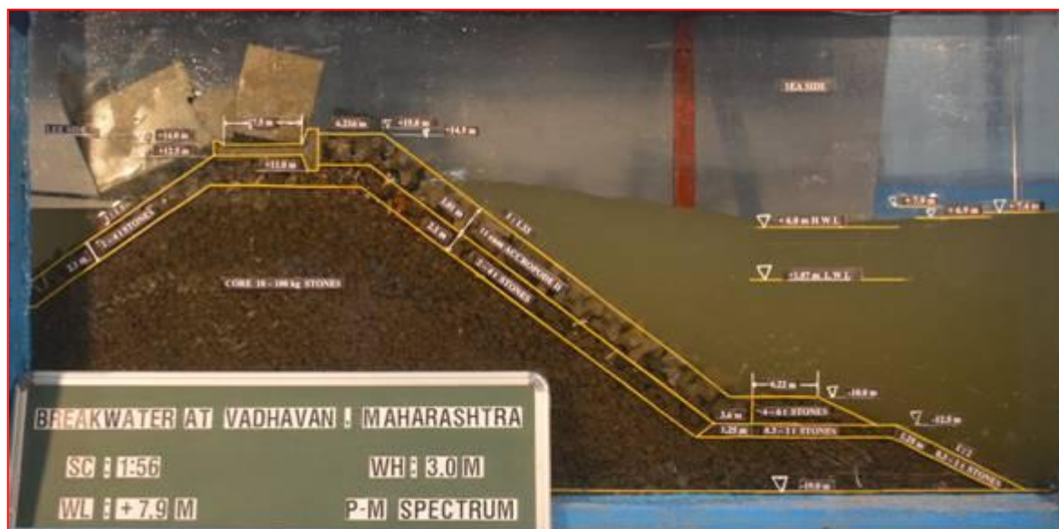
Photo-20: Wave action on trunk section armour layer (11 Cu.m Accropode-II) at -19.0m bed level with wave height of 3.0 m at +7.9 m water level
