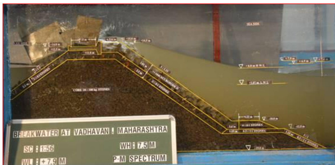
Photo-17: Wave action on trunk section armour layer (11 Cu.m Accropode-II) at -19.0m bed level with wave height of 7.5 m at +7.9 m water level
