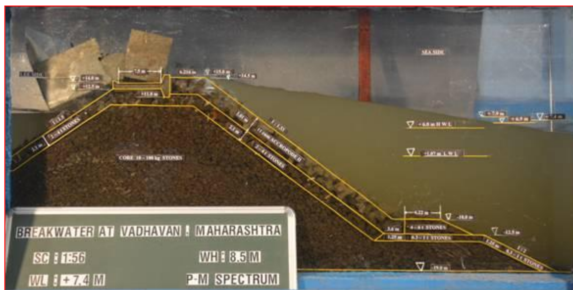
Photo-20: Wave action on trunk section armour layer (11 Cu.m Accropode-II) at -19.0m bed level with wave height of 3.0 m at +7.9 m water level
