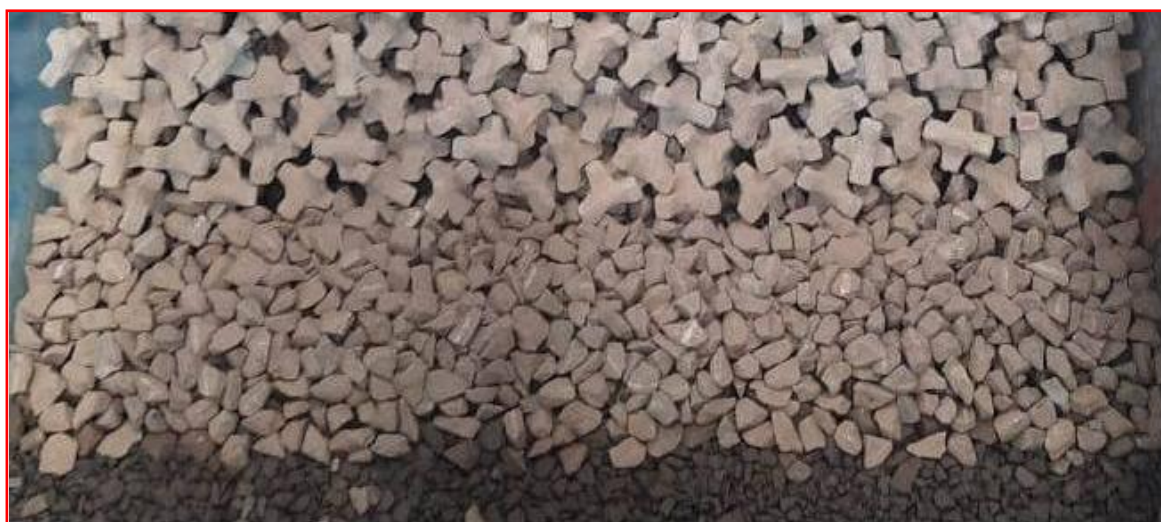
Photo-30: Toe-berm portion of breakwater section before wave generation
