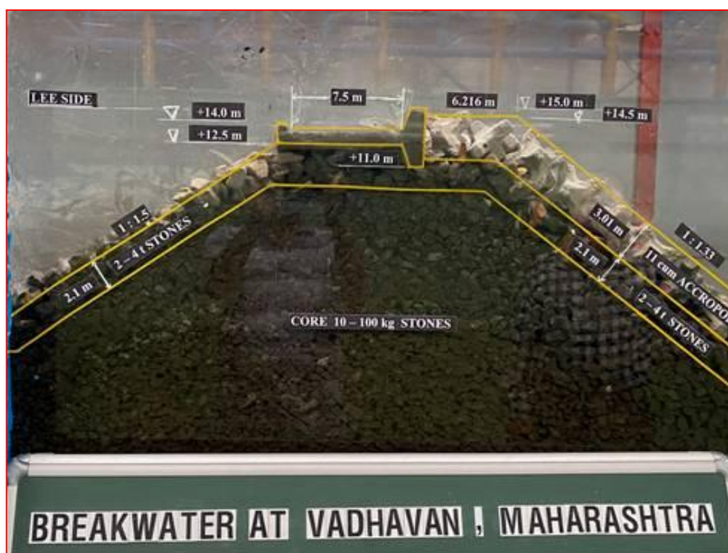
Photo-24: Placement of 2 to 4 t stones on leeside of breakwater section in the wave flume before wave generation
