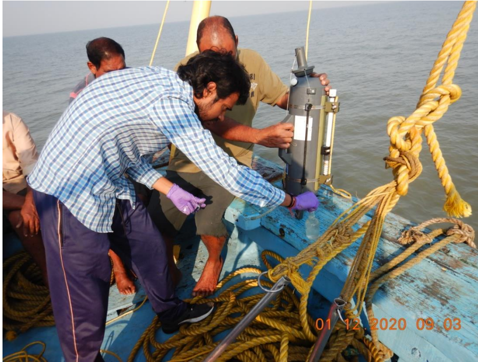
Plate 1: Photo showing collection of bottom water sample using Niskin sampler
