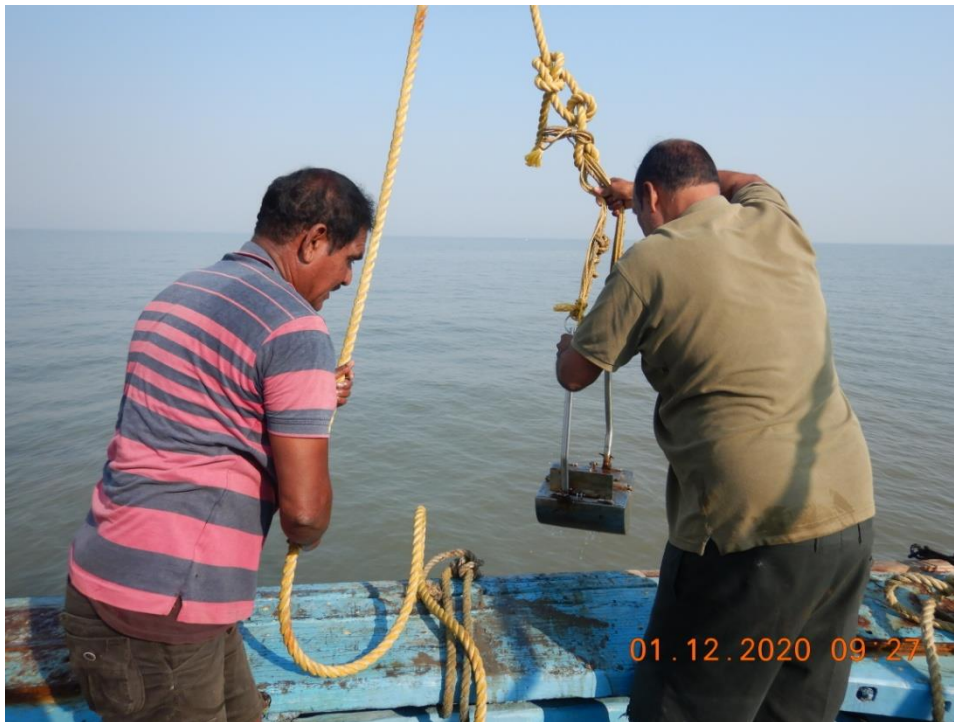
Plate 1: Photo showing collection of bottom water sample using Niskin sampler
