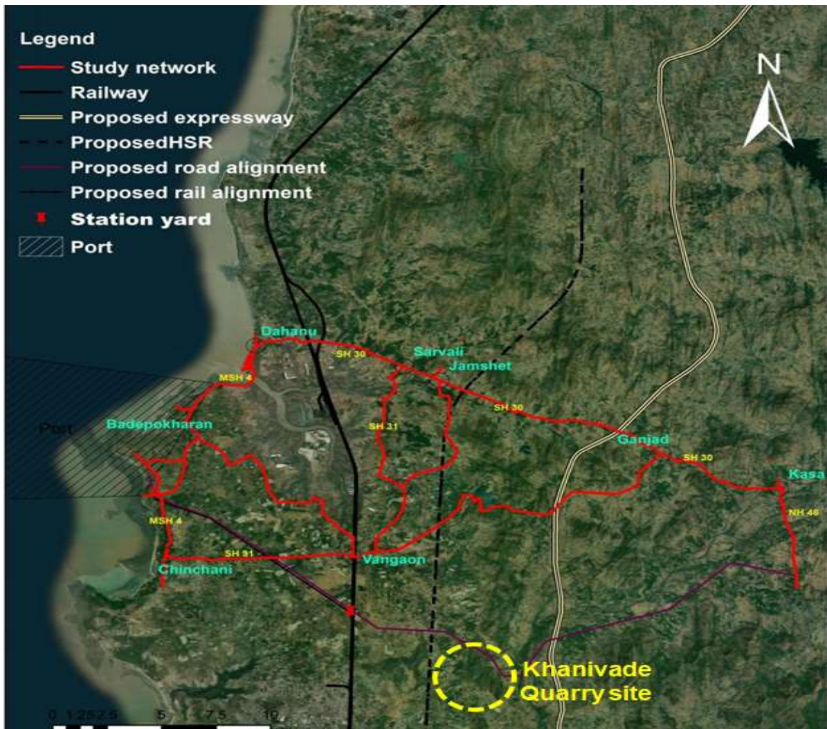
Figure 57 Proposed Road alignment for the Vadhavan port with reference to Khanivade Quarry
