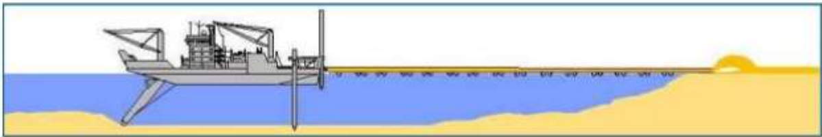
Figure 21 CSD Discharging Onshore through Floating Pipe
