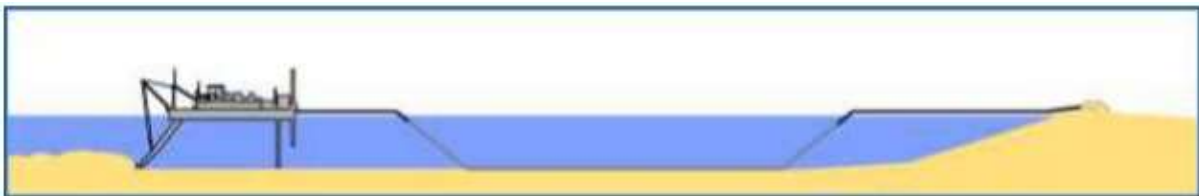
Figure 22 CSD Discharging Onshore through Submerged Pipe
