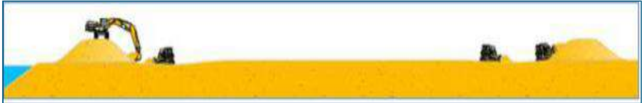
Figure 9-2 Typical Cross section of Raising of the Bunds by using Bulldozers/ Excavator
