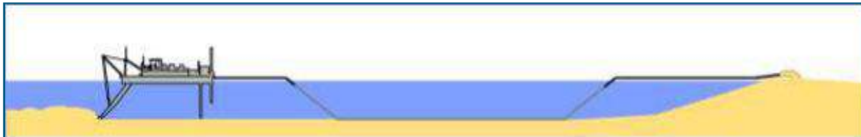
Figure 8-28 CSD Discharging Onshore through Submerged Pipe
