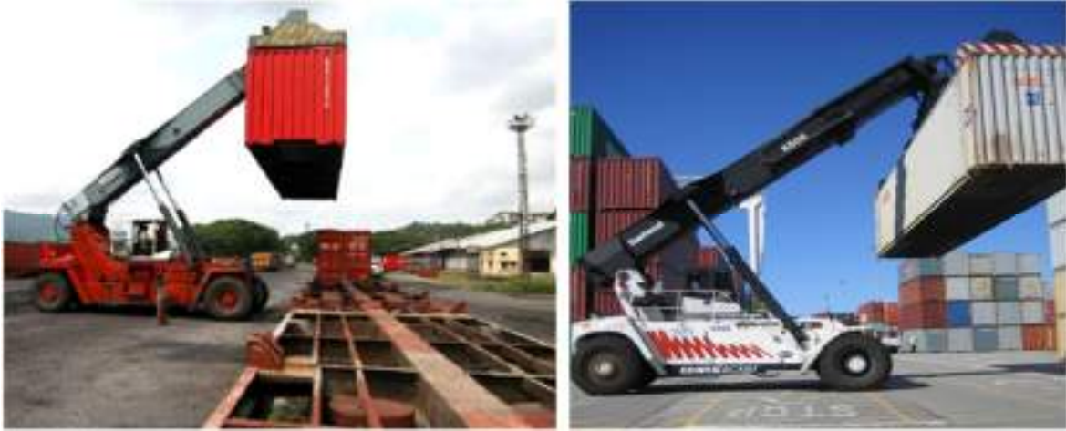
Figure 7-10 Snapshot of Typical Reach Stacker Handling
