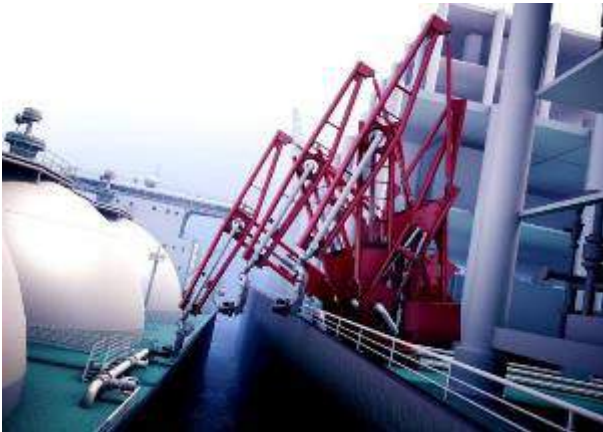
Figure 7.15 LNG unloading Arms (OLFA) designed for offshore applications as LNG
