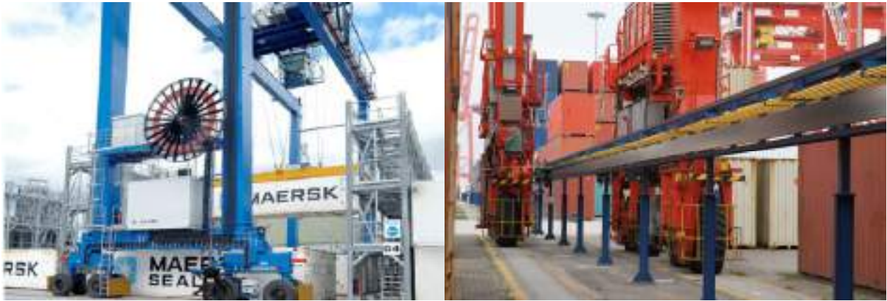
Figure 7-5 Typical E-RTG for Yard Operation with Electric Buss Bar Arrangement for E-RTG
