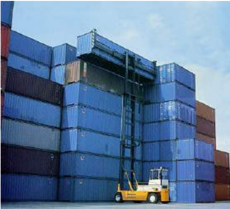
Figure 7-9 Snapshot of Typical Side-pick Handling
